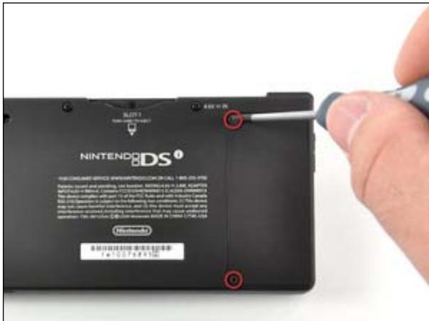
Two Phillips screws prevent access to the battery, unscrew and remove the battery.
