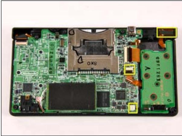
Removing the battery PCB is a pretty straightforward procedure, disconnect three connections and remove the five Phillips screws.
