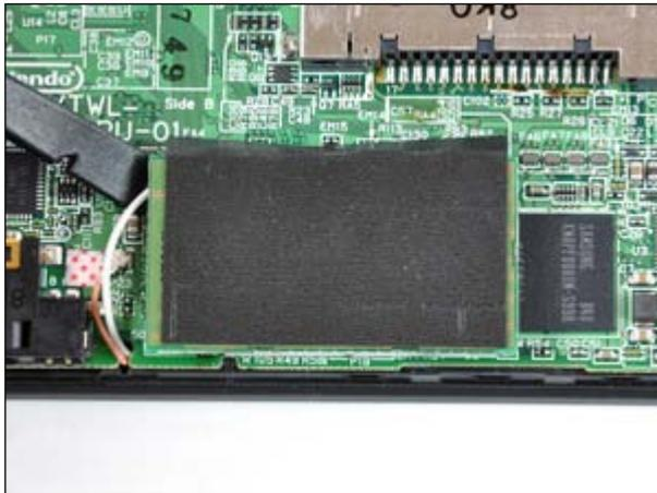
The Wi-Fi board is a push fit into the motherboard socket and pulls off easily, and don't forget to disconnect the Wi-Fi board's connector wire.
