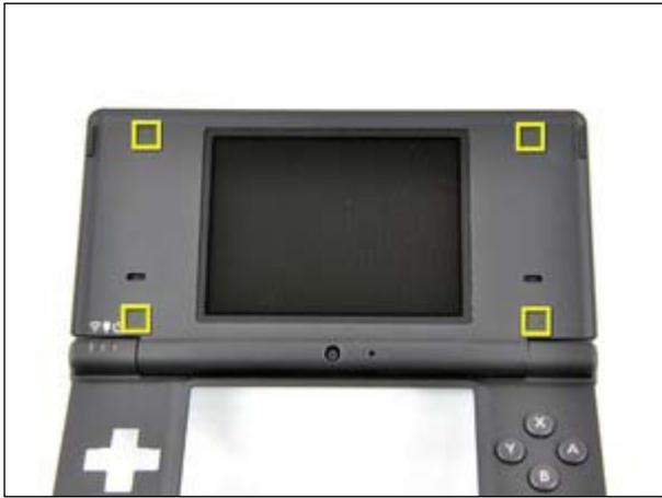
Four plastic covers need to be removed to reveal the Phillips screws underneath. Removing the four Phillips screws allows access to the top display.
