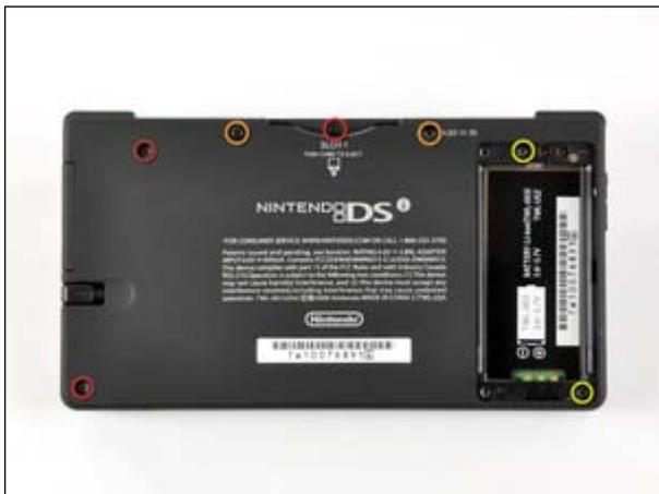
There are a total of seven screws that hold the lower case of the DSi together. Three are immediately visible without removing any plug or cover. Two rubber feet/plugs near the top of the unit have to be removed to reveal two more screws. The inside battery compartment there two additional screws that need to be removed.
