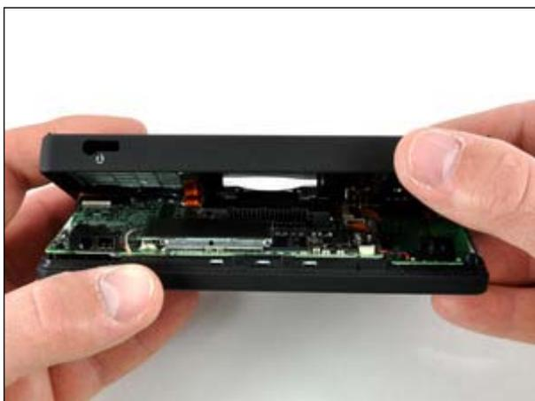
Now the bottom case shell can be removed, an orange connector joins the cases together. Care should be taken when opening the DSi to ensure this connector is not damaged in the process.
