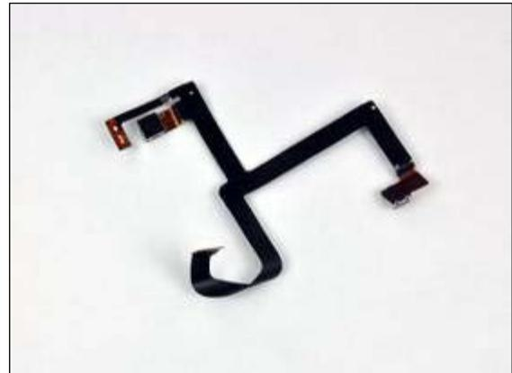
The DSi camera ribbon cable has two VGA CMOS digital cameras (0.3 megapixels); one on the internal hinge pointed towards the user and the other in the outer shell.
