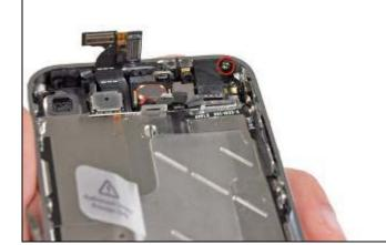
Remove the 1.5 mm Phillips screw securing the front panel near the headphone jack.
