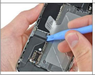
Use an iPod opening tool to gently pry the dock cable connector up off the logic board from both short ends of the connector.
