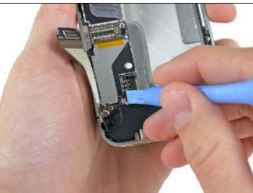
Use an iPod opening tool to pry the lower antenna connector up off its socket on the logic board.
