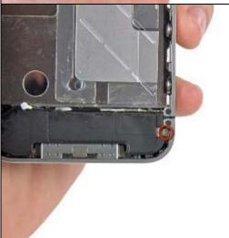
• Remove the single 2.4 mm Phillips screw securing the speaker enclosure to the side of the inner frame.
