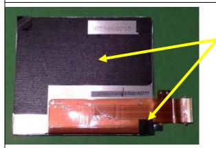
Unfasten the clip holding the LCD screen ribbon cable and remove the cable.
