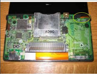
This is the clip for the upper screen, (circled on main photo to left) use a small flat head screwdriver to gently open it.
