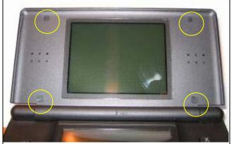
Remove the square rubber screw covers with a small flat head screwdriver or craft knife. Remove the 4 x posidrive screws. (Photo left)
