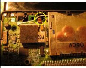
Unfasten the clip holding the touch screen ribbon cable and remove the cable. Please note that the clip opens from the back and NOT the front.
