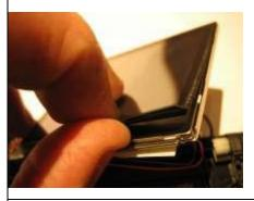
The LCD has a seal which has to be removed from the old screen to use on the new. (photo left)
