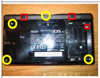
Next remove the 4 tri-head screws (circled) and the 3 cross-head screws. 2 of the cross head screw are hidden under the 2 small rubber feet. The rubber feet pick out with a small screwdriver and have sticky adhesive so keep to one side to stick back in at the end.
