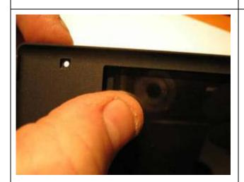
With the top cover removed, open the top up as if you are going to play on it, then gently push out the LCD unit from the casing starting at the top corner. (photo to left)
