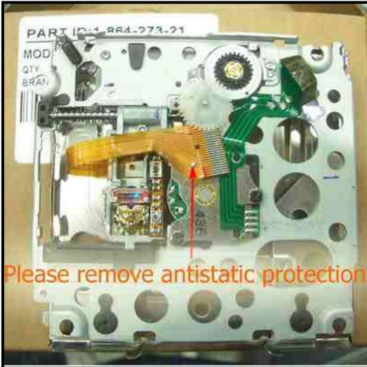
1<sup>st</sup> job is to remove the antistatic bridge solder blob. (Use a low wattage soldering iron and a solder removal tool for best results)
